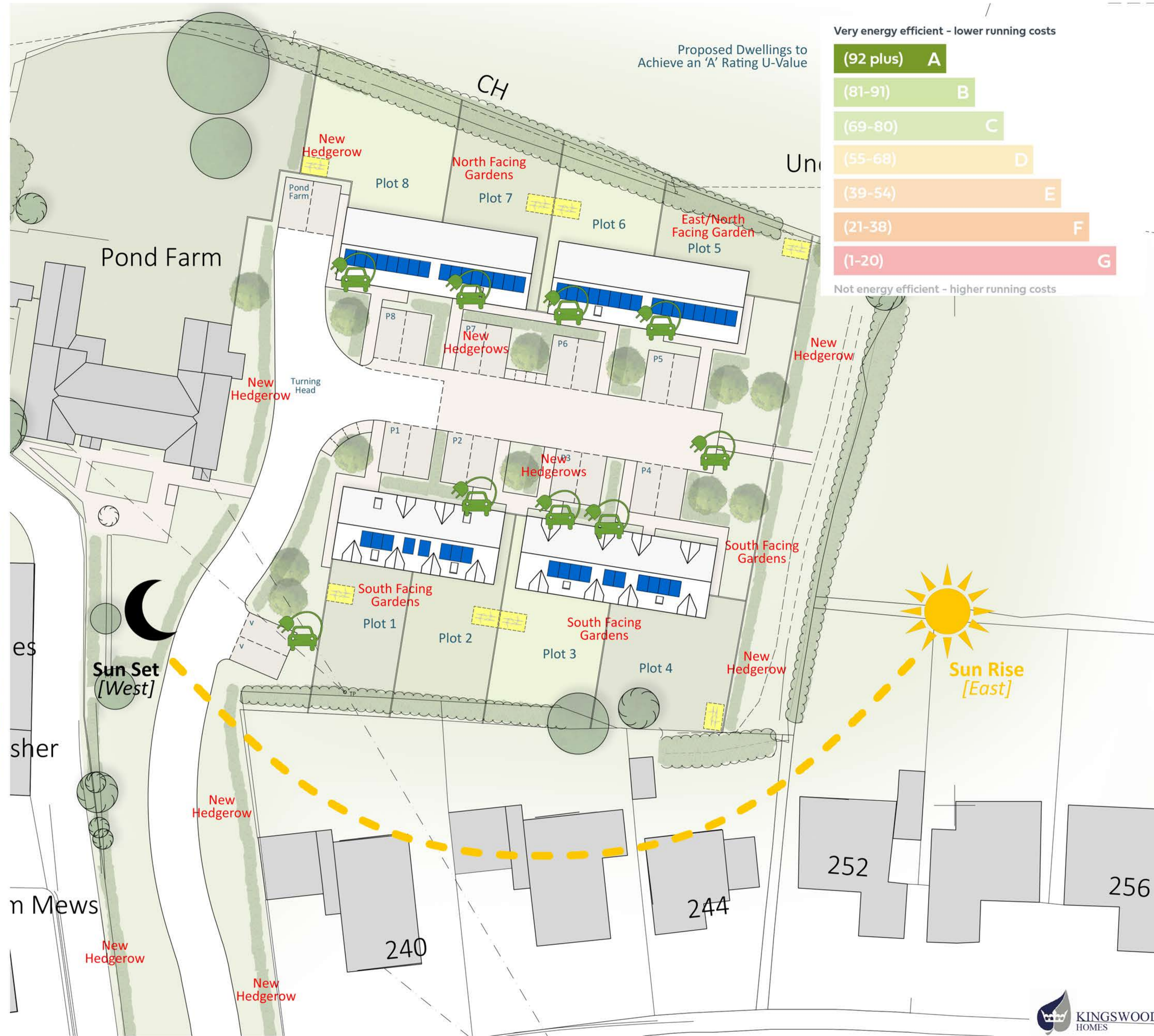
Photo Voltaic Panels [PV]. The Houses Have Been Orientated With South Facing Pitched Roofs [East/West For Plot 5] to Incorporate PV Panels.
