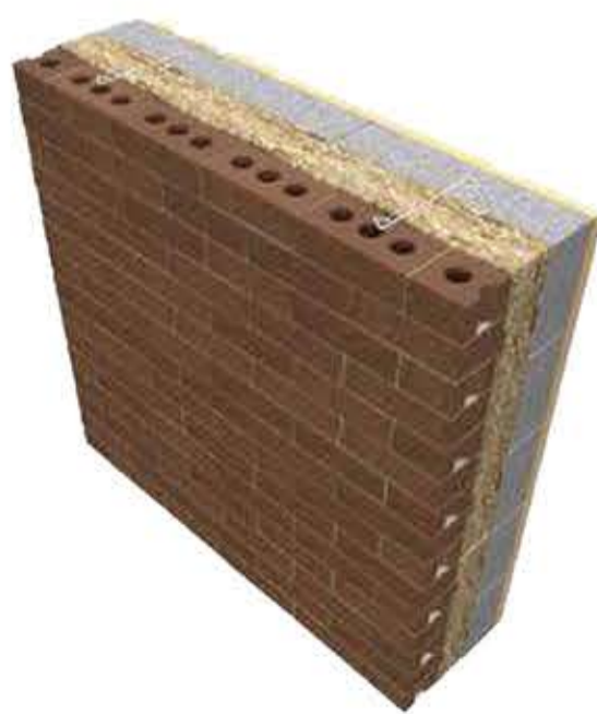
Enhanced Insulation - Each House Will Incorporate Enhanced Levels of Insulation to Comply With New Part L Building Regulations 2023
